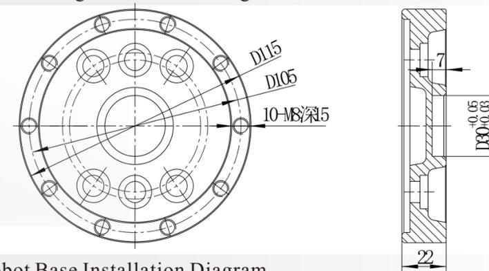
Robot Base Installation Diagram
